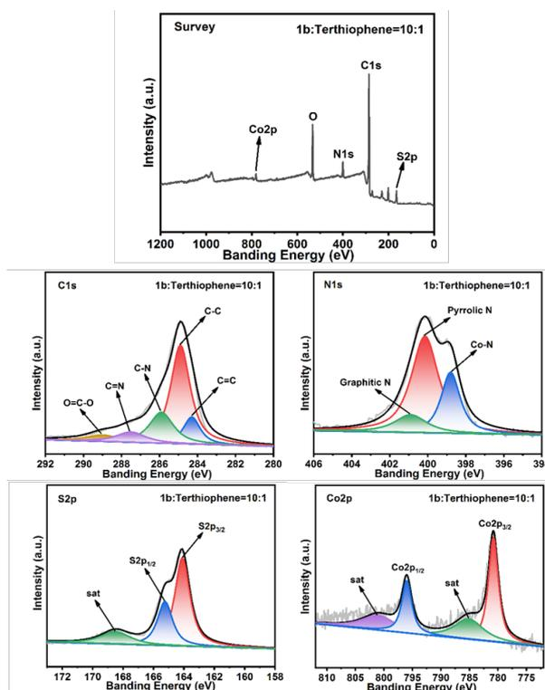
**Figure 4** The XPS analysis of Co<sup>III</sup>corrole-trithiophene conductive polymer modified carbon paper.
