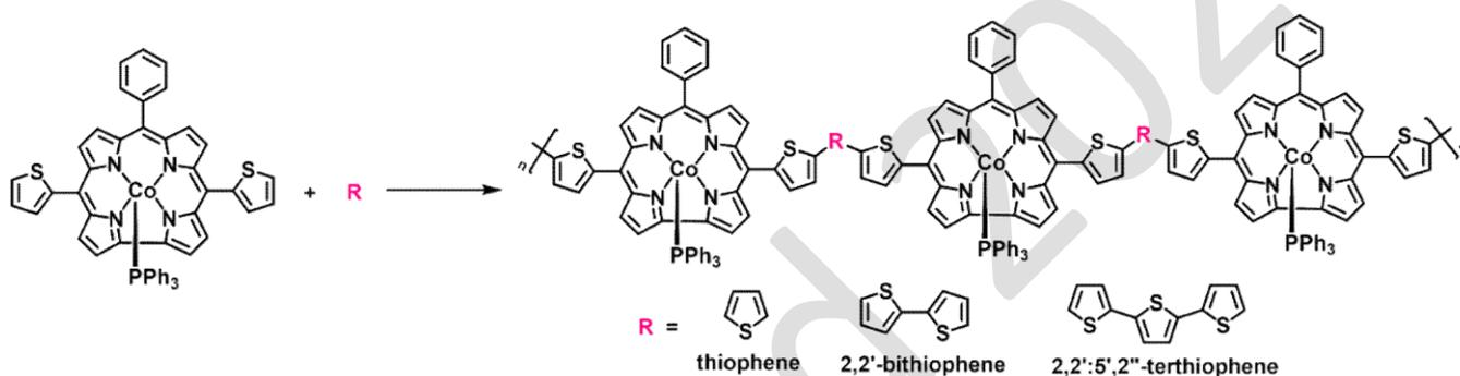
**Scheme 1** The synthesis of Co<sup>III</sup>corrole **1b** copolymerized with mono-, bis- and tri-thiophenes.
