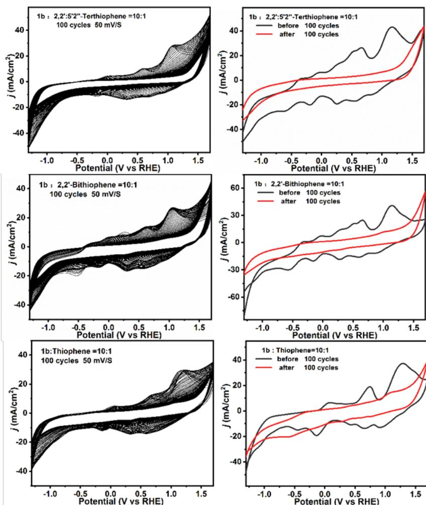
**Figure 1** The CV polymerization curves of Co<sup>III</sup> corrole **1b** copolymerized with mono-, bis- and tri-thiophene (left) and CV comparison chart before and after 100 cycles electropolymerizations (right).
