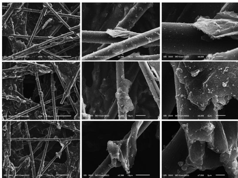
**Figure 2** The SEM images of Co<sup>III</sup>corrole **1b** copolymerized with mono- (first row), bis- (second row) and trithiophene (third row) modified carbon papers.
