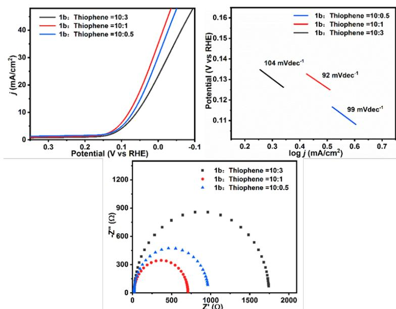
**Figure 7** LSV plot, Tafel slope and EIS diagram of Co<sup>III</sup>corrole **1b** copolymerized with thiophene in different molar ratios modified carbon papers.
