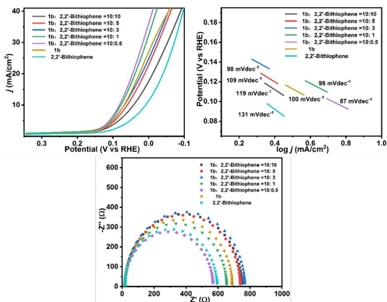
**Figure 5** LSV measurements, the calculated Tafel slope and EIS diagram of Co<sup>III</sup> corrole-bisthiophene copolymers with different molar ratios modified carbon papers.
