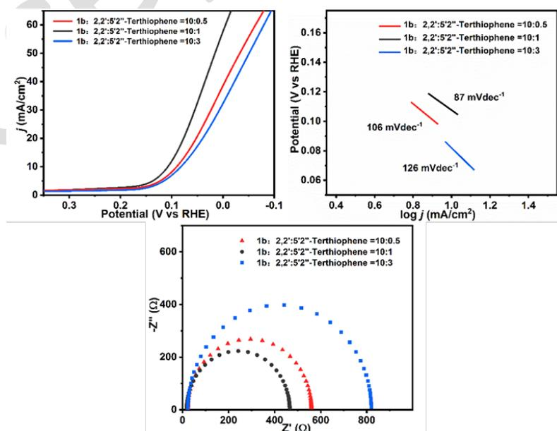
**Figure 6** LSV plot, Tafel slope and EIS diagram of Co<sup>III</sup>corrole **1b** copolymerized with 2,2':5'2''-terthiophene in different molar ratios modified carbon papers.
