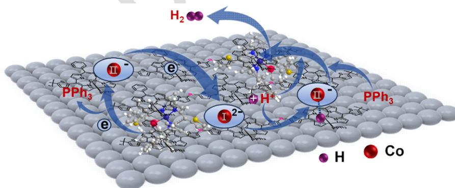
**Figure 9** Catalytic hydrogen evolution mechanism of  $\text{Co}^{\text{III}}$ -corrole **1b** copolymer conductive polymer.
