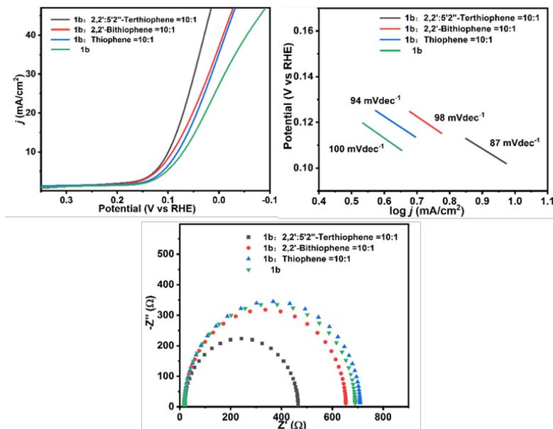
**Figure 8** LSV plot, Tafel slope and EIS diagram of  $\text{Co}^{\text{III}}$ corrole **1b** and three thiophenes in a molar ratio of 10:1 modified carbon papers.
