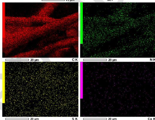
**Figure 3** The EDS mappings of Co<sup>III</sup>corrole-trithiophene conductive polymer modified carbon paper.
