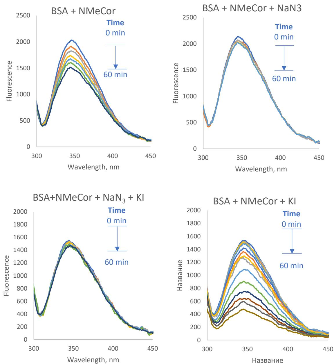
**Figure S6.** Corrected fluorescence spectra upon irradiation of a complex of BSA (0.08 wt %) with NMeCor ( $1.7 \cdot 10^{-5}$  M) depending on the presence of KI (50 mM) and NaN<sub>3</sub> (15 mM).
