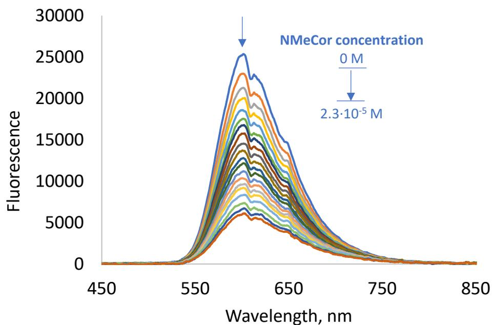
**Figure S2.** Fluorescence spectra ( $\lambda_{\text{ex}}=295$  nm) of titration of DNA ( $1.1 \cdot 10^{-4}$  M)-EtBr ( $1.3 \cdot 10^{-5}$  M) complex with **NMeCor**. Titration was performed by adding of **NMeCor** (0.45 mM) 5  $\mu$ l (19 steps) to 2 ml of DNA-EtBr complex in Tris-HCl buffer in a cuvette with stirring at a temperature of 25  $^{\circ}$ C.
