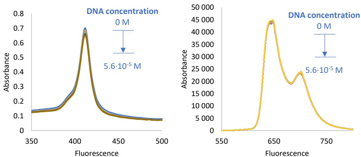
**Figure S1.** UV-Vis and fluorescence ( $\lambda_{\text{ex}}=425$  nm) spectra of **pSCor** during titration with DNA. Titration was performed by adding DNA (1.6 mM) 10  $\mu\text{l}$  (7 steps) to 2 ml of corrole solution in Tris-HCl buffer in a cuvette with stirring at a temperature of 25  $^{\circ}\text{C}$ .
