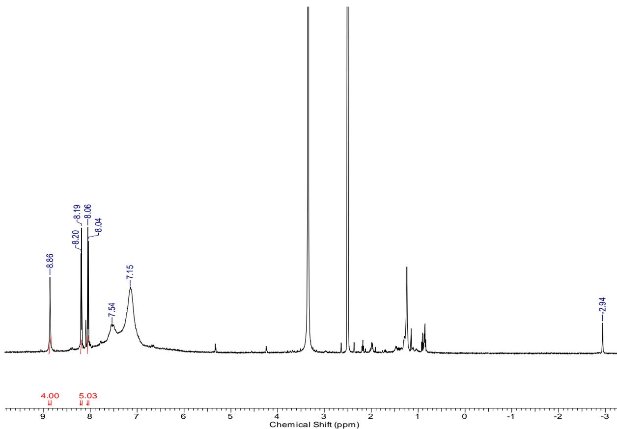
$^1\text{H}$  NMR spectrum of a mixture of tri- and tetrasulfophenylcorroles
