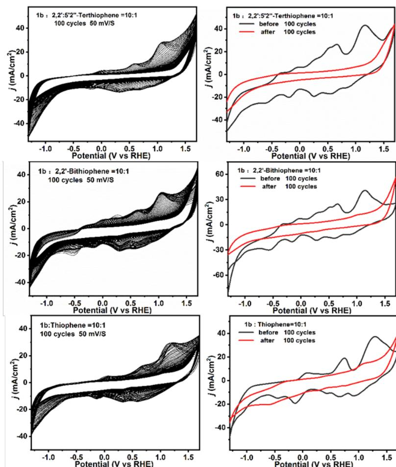
**Figure 1.** The CV polymerization curves of Co<sup>III</sup>corrole **1** copolymerized with mono-, bis- and tri-thiophene (left) and CV comparison chart before and after 100 cycles electropolymerizations (right).
