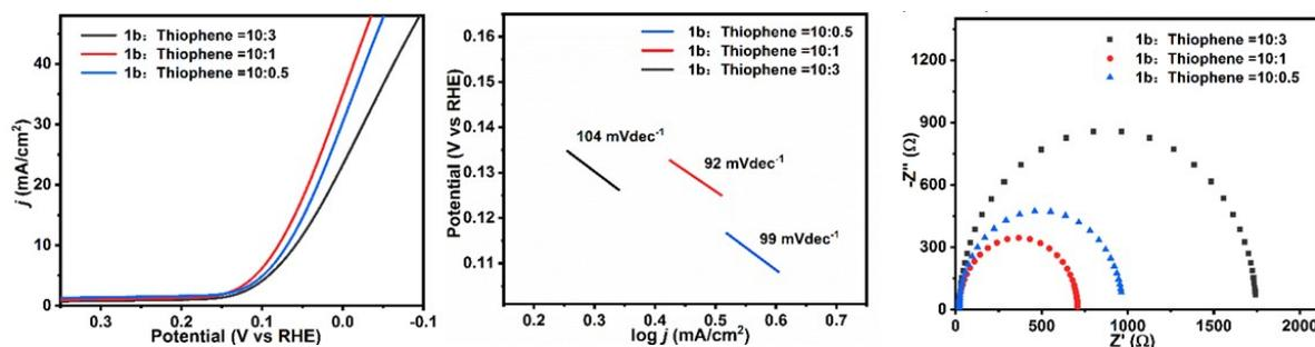
**Figure 7.** LSV plot, Tafel slope and EIS diagram of Co<sup>III</sup>corrole 1 copolymerized with thiophene in different molar ratios modified carbon papers.
