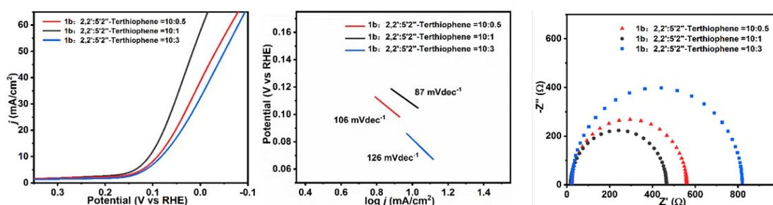
**Figure 6.** LSV plot, Tafel slope and EIS diagram of Co<sup>III</sup>corrole 1 copolymerized with 2,2':5'2''-trithiophene in different molar ratios modified carbon papers.
