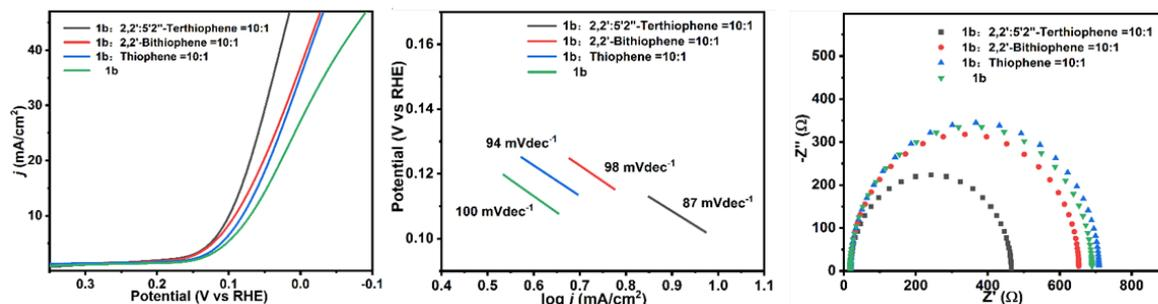
**Figure 8.** LSV plot, Tafel slope and EIS diagram of Co<sup>III</sup>corrole 1 and three thiophenes in a molar ratio of 10:1 modified carbon papers.
