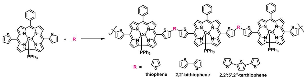
**Scheme 1.** The synthesis of Co<sup>III</sup>corrole **1** copolymerized with mono-, bis- and tri-thiophenes.
