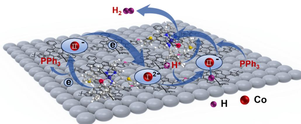
**Figure 9.** Catalytic hydrogen evolution mechanism of Co<sup>III</sup>-corrrole **1** copolymer conductive polymer.
