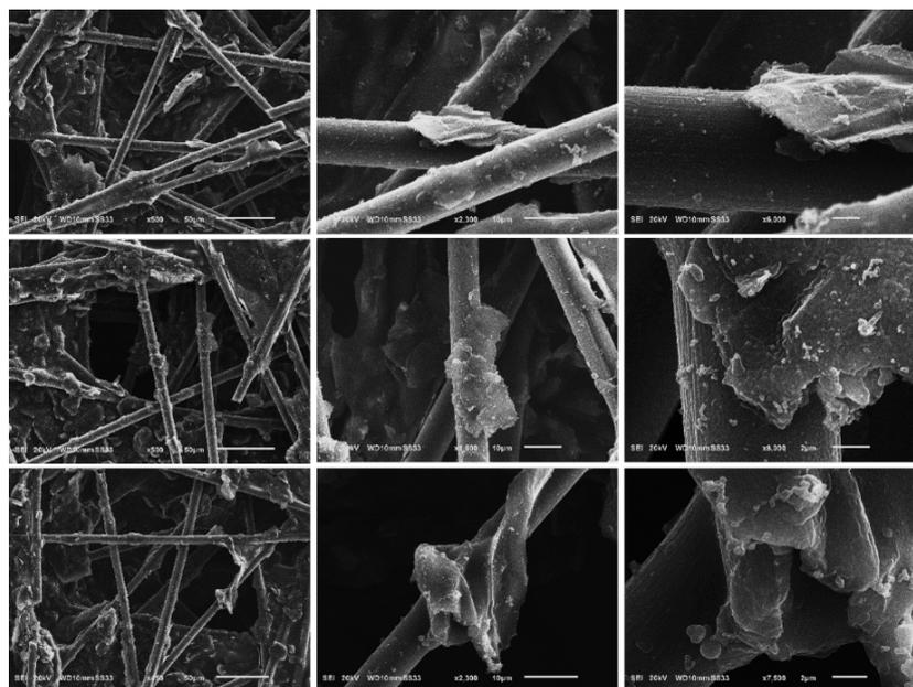
**Figure 2.** The SEM images of Co<sup>III</sup>corrole **1** copolymerized with mono- (first row), bis- (second row) and trithiophene (third row) modified carbon papers.
