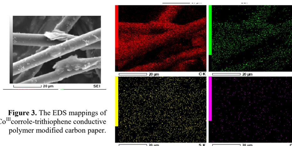
**Figure 3.** The EDS mappings of Co<sup>III</sup>corrole-trithiophene conductive polymer modified carbon paper.
