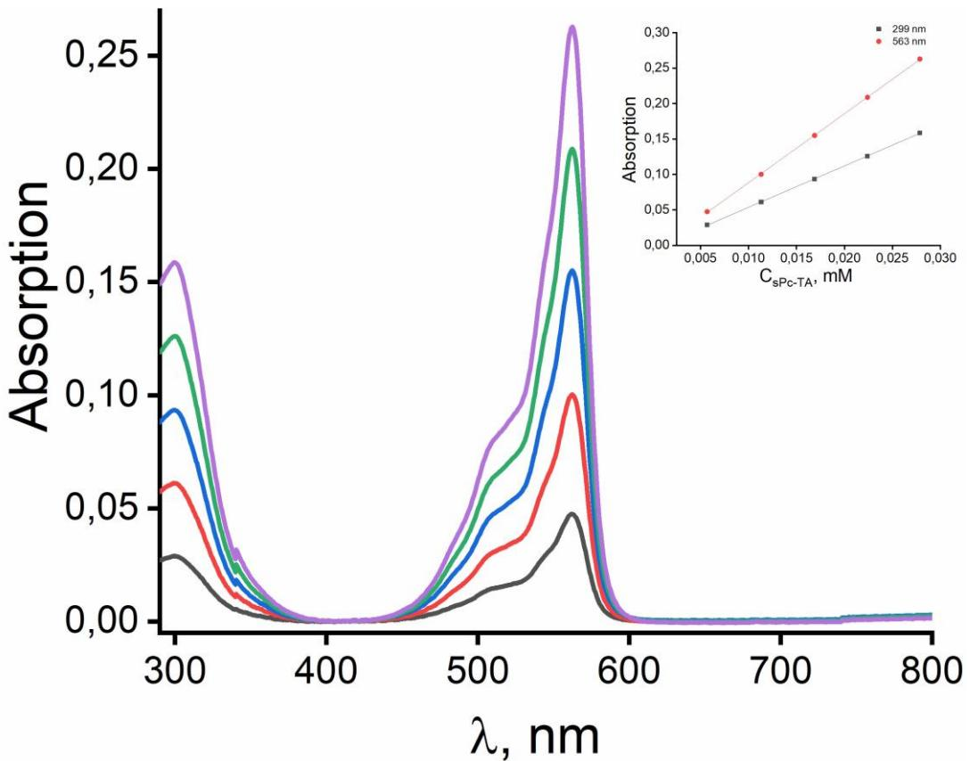
**Fig. S. 42.** Electronic absorption spectra of **sPcTA** in EtOH at different concentrations. Dependence of concentration on optical density is shown in the inset
