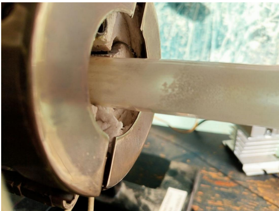
Figure 1. Fragment of the glass reactor tube after synthesis
